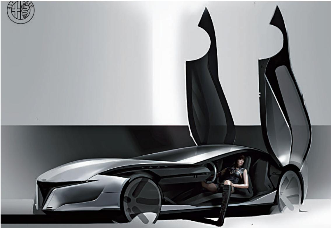
A sketch that illustrates the research done for the doors, designed to ease access and at the same time make the opening spectacular. Hence the hinged door panels on the rear wheelarch that lift vertically upwards to reach a height of 3643 mm.
