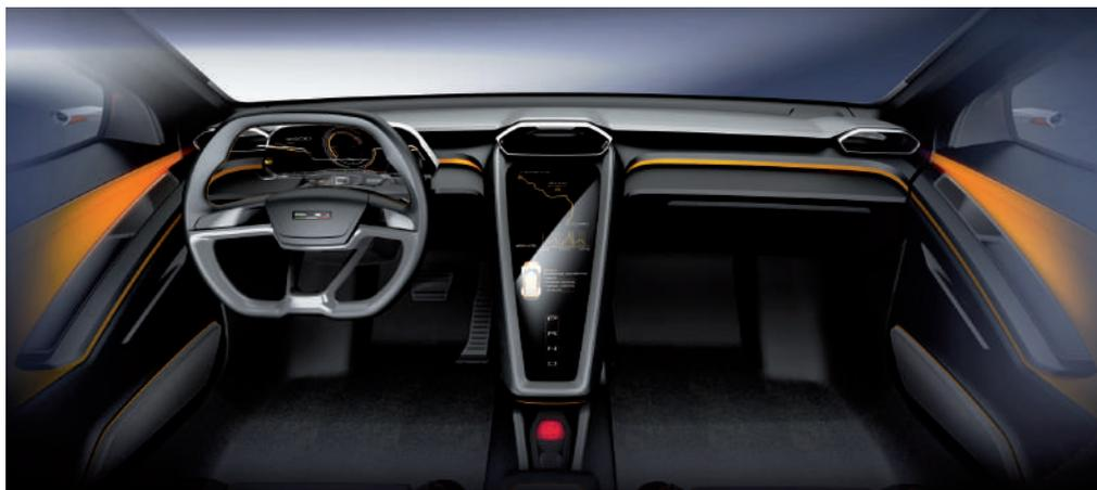
All buttons (with the exception of the parking brake control) have been done away with and replaced by a large screen extending down into the centre console. This display uses multi-touch technology, with different settings and menus displayed depending on how many fingers are placed on the screen.
