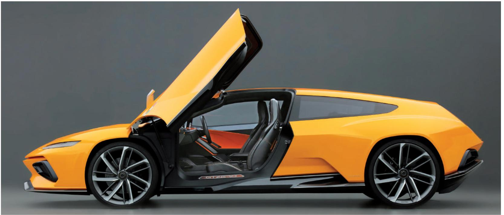
The scissor doors also include a portion of the roof to make getting in and out of the car more comfortable. Below, a view of the dash, with its minimalist, sophisticated design.
