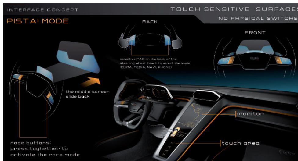
A study rendering for the interior, with its comfortable, cocooning architecture. The cabin has room for four, with seats in 2+2 or 3+1 configurations. Opposite, the two different drive modes: 'Drive' and 'Pista!' (track), selected from pads behind the steering wheel – which doubles up as the main control console of the car.
