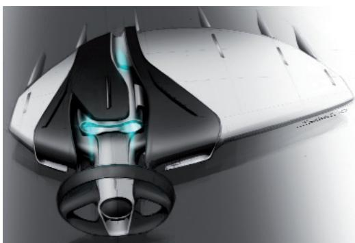
Left and below, more sketches by Pierre Sabas and Alister Whelan illustrating the futuristic and evolved character of the concept. The dash has a floating design and is made from premium materials. It moves together with the pedal box as the seats are fixed.
