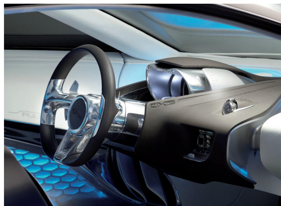
The interior of the concept. The smooth, fluid curves, explains Callum, were inspired by the flow of air into the turbines. Note the electroluminescent microfilaments and the phosphor blue LEDs.
