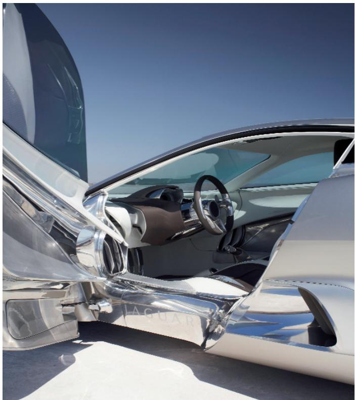
The finished C-X75: note the huge air intakes in the flanks for the microturbines and the lack of exhaust pipes at the rear. The rear screen is reminiscent of the E-type.
