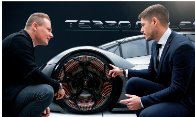
Electric motors are fitted in each wheel and the particular design aims to express their power. In the photo, Borkert and Facundo during the presentation of the car at the MIT in Boston.
