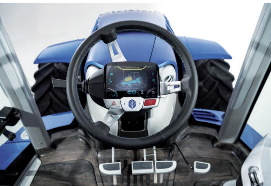
The finished prototype, in the two images above. Left and below, the final solutions for the interior. An important feature is the fixed screen in the middle of the steering wheel.
