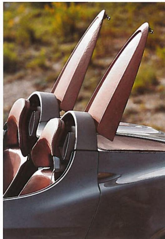
Left, two details of the Tango's rear section with its two luggage compartments set behind the rollbars. Each contains a specially designed "trolley"-type case.
