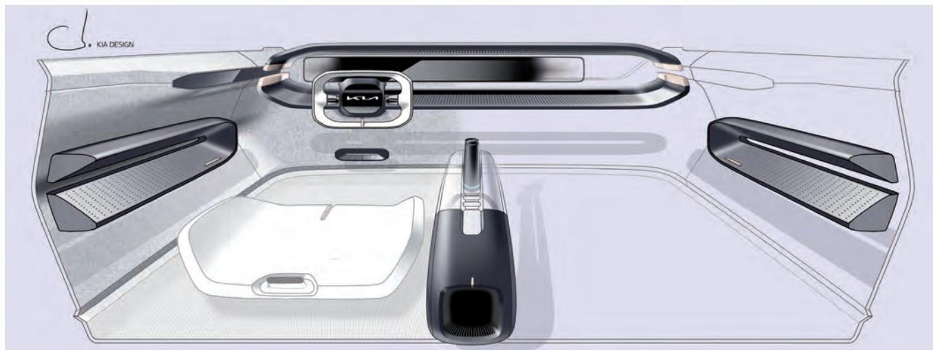
The dashboard has a ring-like structure into which a large screen extends to the centre. It is based on the Technology for Life concept, in other words non-invasive presence of technology. The ventilation slits are linear and concealed.
