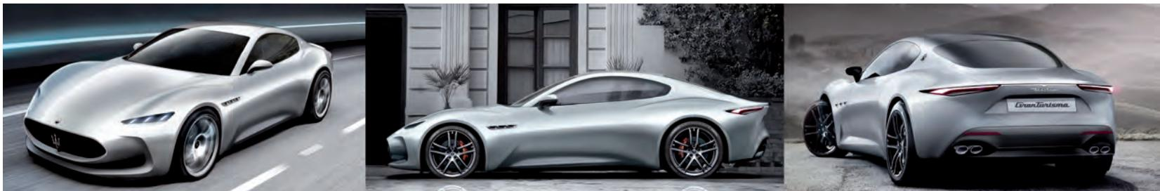
the grille with parallel slats to the Trident positioned on the C-pillar," continues Busse, as he shows us the bonnet, a single piece of aluminium (3.5 square metres of surface area) that covers the 3.0 V6 Neptune engine positioned mid-front (but the GranTurismo also comes in a 100% electric version, the Folgore, with 760 hp).
