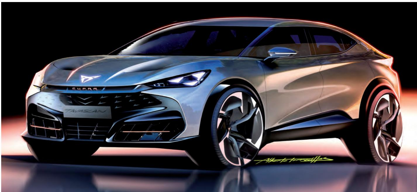
The negative-cut, "shark nose" front end is modelled to optimise aerodynamics, as is the wedge-shaped body in which the side muscles extend to the tail end. The lower air intakes help cool the batteries.
