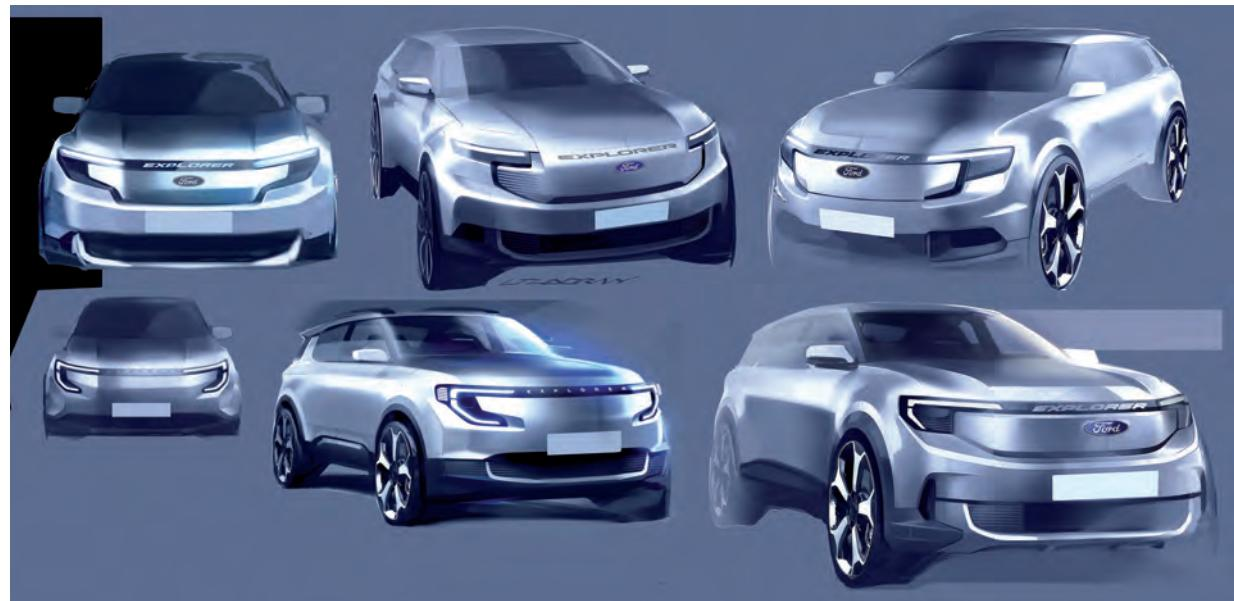
While the nose has undergone fine variations in detail, nowhere did the designers discuss the design of a volume that is visually separated from the passenger compartment and lacks a traditional grille. The bonnet neither opens nor conceals a boot, contributing to the pleasing 'monolithic' effect.
